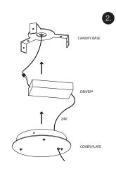
ASSEMBLY WITH DRIVER\* Connect the transformer/driver (220V/110V to 24V\*) to the house electric wire. Pull the low voltage wire coming from the transformer through the canopy cover plate.
