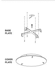
Mark and drill holes in the ceiling based on the base plate size. Carefully unwrap and attach the base plate to the ceiling using dowels and screws (by client).
