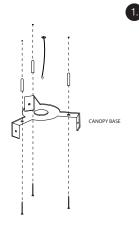
Mark holes in the ceiling based on canopy measurements. Attach canopy base plate using screws and plugs (by client).
