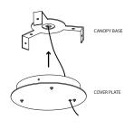
ASSEMBLY WITHOUT DRIVER Pull through cover plate the house electricity cable or connect the lamps electric cable (through cover plate) to the house electricity wire.
