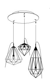
Carefully unwrap the Diamond lights and guide the suspension cables through the cable fasteners located on the cover plate.
