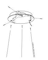
Fix cover plate to the base plate with three included screws. Once tightly fixed proceed to hanging the lamp by guiding the lamps suspension cables through the little nozzles.
