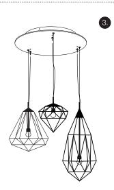
Pull through each Diamonds electric cable through the cover plate.
