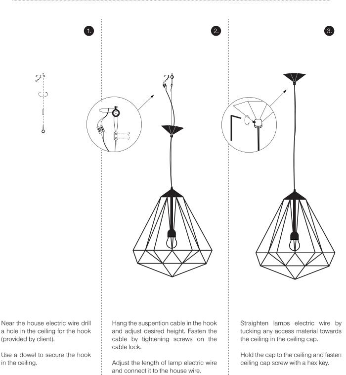
Bulb: E27 fitting max 60W
