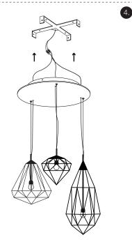
Connect each lamps electricity cable to the house electricity cable and tuck all excess cables inside the cover plate before attaching the cover plate to the base plate.
